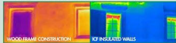
Wood frame walls (left) are warm and lose heat, ICF walls (right) remain neutral losing little to no heat.
